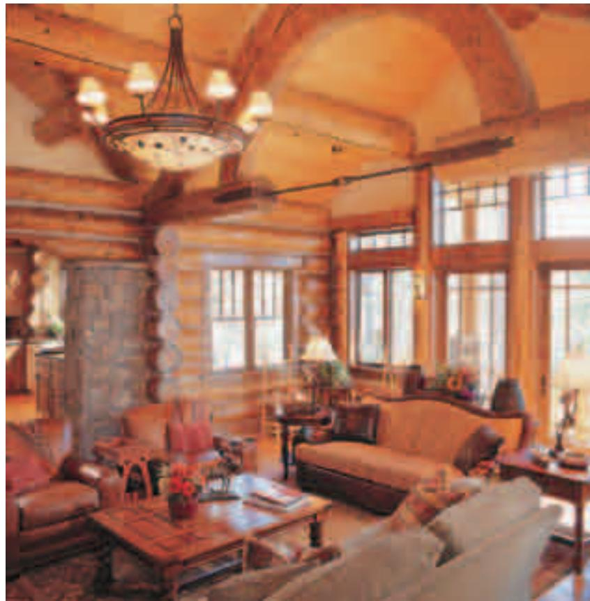
The log walls in the great room have a stone extension to give the appearance that the exterior wall of an original small cabin was cut through to allow for an addition. Architect Ellis Nunn featured a hammer truss and oversized headers over the Pozzi windows. The custom wrought iron chandelier with aspen leaf detail is made of faux rawhide because real rawhide cracks when exposed to the heat from the lights.
